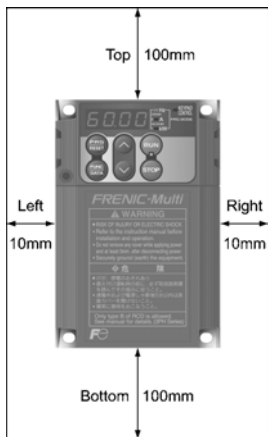
Figure 2.1 Mounting Direction and Required Clearances
